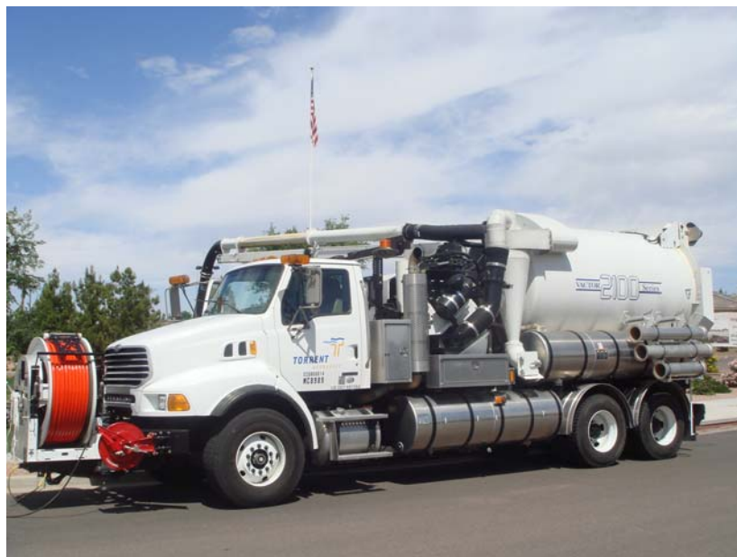
Typical Hydrovector Truck used for Drywell Maintenance
