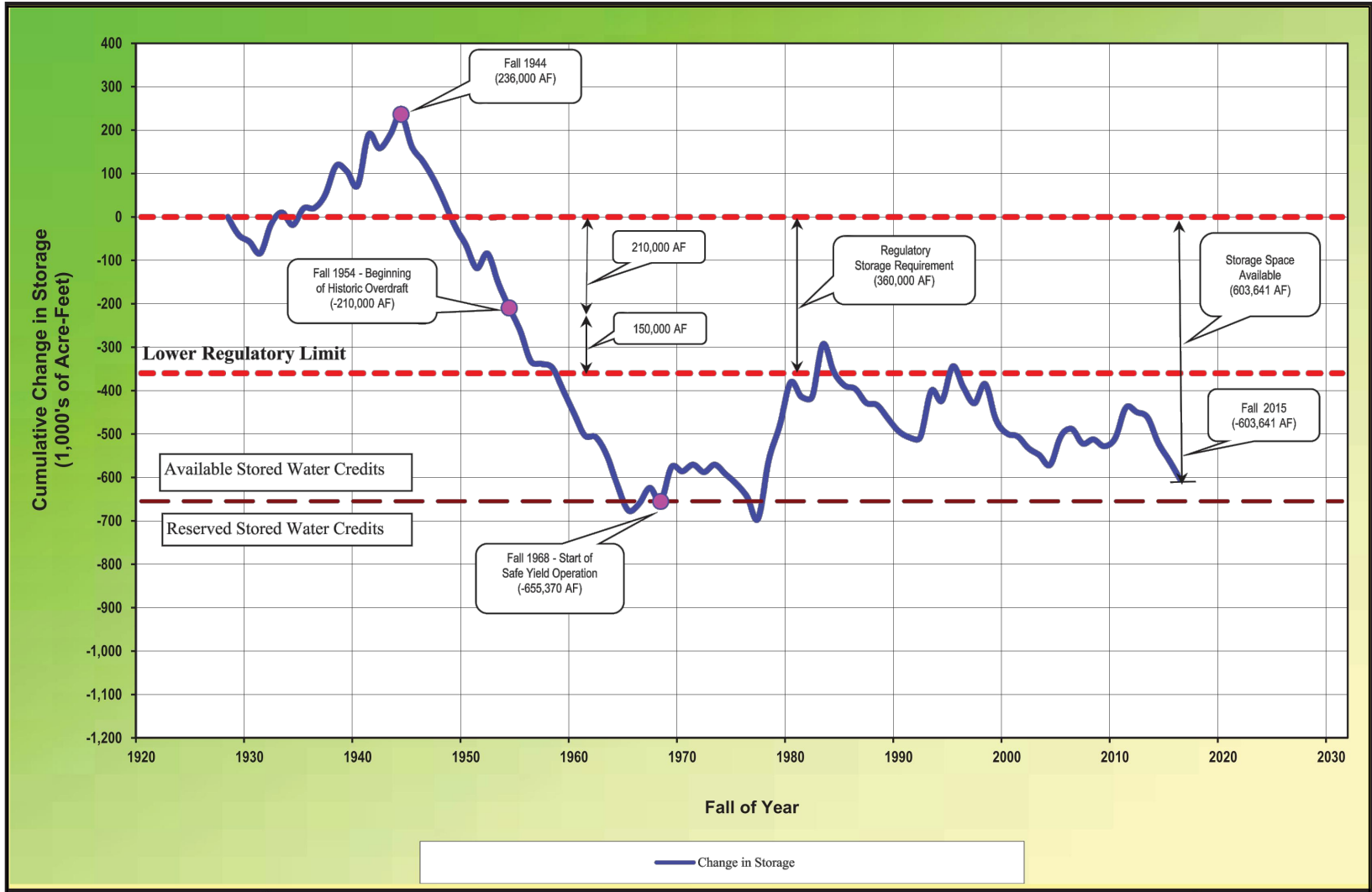
2015-16 Water Year ULARA Watermaster Report San Fernando Basin: Cumulative Change in Groundwater Storage PLATE 7
