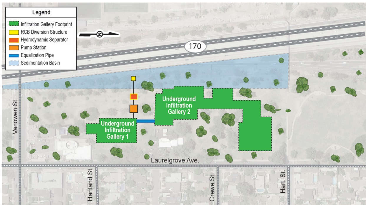
Figure 1 Project North Subsurface Stormwater Project Features
