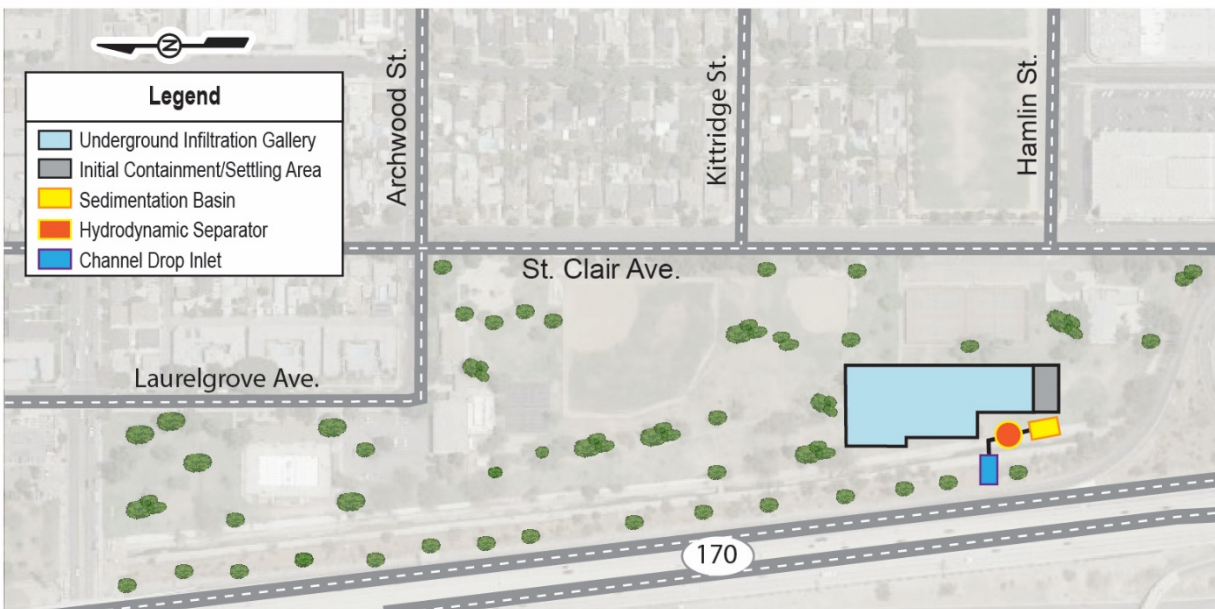
Figure 2 Project South Subsurface Stormwater Project Features
